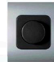
DIMMER FOR INCANDESCENT LAMP WITH PUSH ON PUSH OFF SWITCH For flush mounting 60 - 500W 220V~ Article B191 (one way) Article B191/2W (two way/change over)
