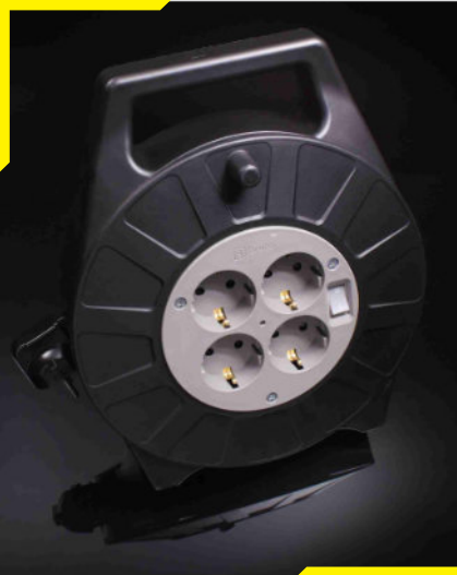
CABLE ROLL extension 10 meters length with switch, 4 socket Art. 15721-10 Rating 250V~, 1000W - 2500W / 10A max
