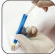
Put into handle kerosene or other suitable lubricants and screw tight cover
