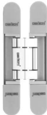
CONCEALED HINGE ES CONC D80 NA Available : Matt Black Capacity (max) : 80 KG / pair Max. Door Width: 90 cm Opening Angle : ≤ 150°
