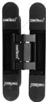
CONCEALED HINGE ES CONC D40 MATT BLACK Available : NA Capacity (max) : 40 KG / pair Max. Door Width: 80 cm Opening Angle : ≤ 150°
