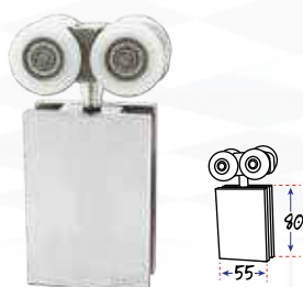
Hanger Rafes RDG TH 5700~sn Type : SP 8204 Material : Stainless Steel Sus 304 Max Weight : 80 kg/door leaf
