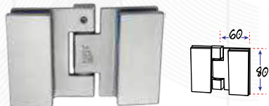
Glass Door Hinge RSH 850H~sn Type : APL 0003 Material : Stainless Steel Sus 304 Max Weight : 80 kg/door leaf
