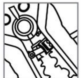
Cut 10-30 AWG (0.05-6mm 2 )
