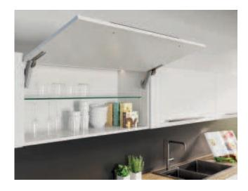
> Area of application: For heavy stay flap applications up to 15 kg (with cabinet height 600 mm) Housing: Plastic. > Material: front fixing bracket and support lever: Steel Front fixing bracket: Nickel plated, > Finish/colour: support lever: Nickel plated or black (with black housing), housing: White, light grey, anthracite or black > Opening angle: 90° or 107° Adjustment facility: Height, side, tilting angle, holding power
